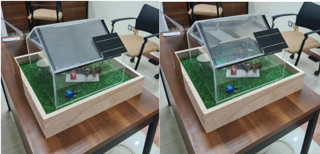
Figure 4. Implementation of the system: PDLC is on one the left and PDLC is transparent on the right
