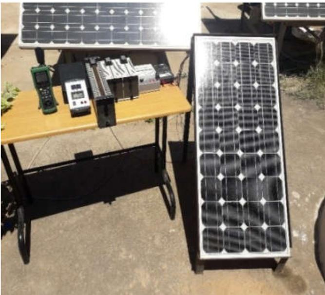
Fig. 2. Test bench to determinate the electrical characteristics.
