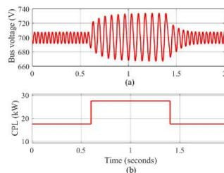
Fig.11 DCMG parameters without CESS; a) DC bus voltage, and b) CPL
