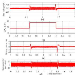
Fig.12 DCMG parameters with CESS; a) DC bus voltage, b) CPL, c) Battery current, and d) Supercapacitor current
