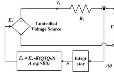
Fig. 4 Simplified nonlinear circuit model of battery.
