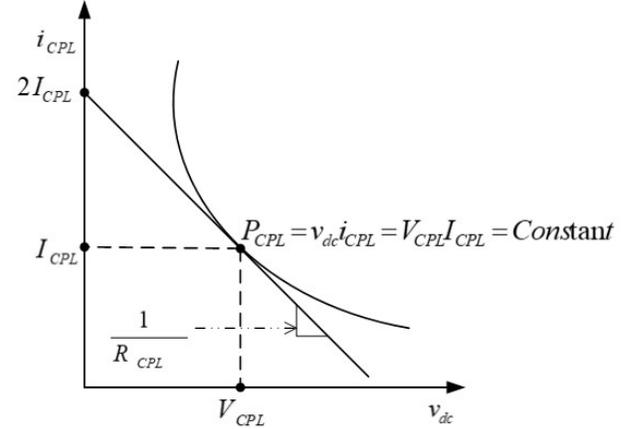
Fig. 2 Current-voltage characteristics of constant power load
