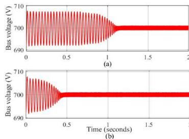
Fig.10 DC Bus voltages with a combination of CPL and resistive load; a) 9.5 kW CPL with 8 kW resistive load, and b) 8.75 kW CPL with 8.75 kW resistive load.
