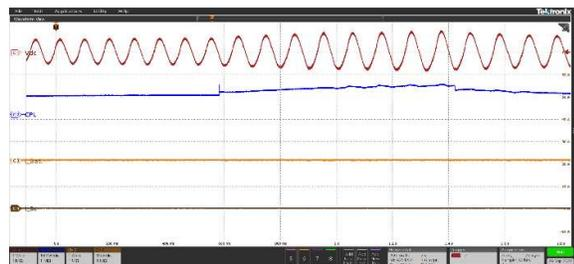
result. Figure 16c2 represents the CPL, whereas Figure 16c3 and 16c4 shows battery and supercapacitor current currents, respectively. In the process of mitigation of instability, both battery and supercapacitor carry ripple current with zero average value. The battery is sensitive to this ripple current, but its peak-to-peak magnitude is less than 2 A which is not so severe, whereas, for the supercapacitor, it's 40 A and bearable.
