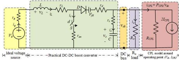
Fig. 3 Practical DC-DC boost converter interfaced with CPL and resistive load.
