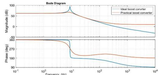
Fig. 8 Bode plots of control output functions of ideal and practical DC-DC
