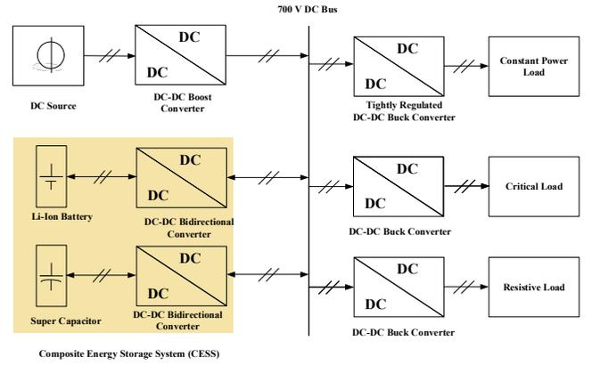
Fig. 1 Configuration of DCMG feeding CPL and resistive load with CESS
