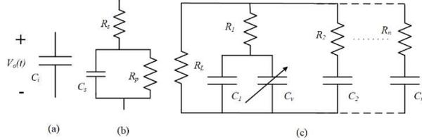
Fig. 5 Equivalent models of supercapacitor: (a) Capacitor under ideality ( $C_i$ ), (b) Simplified model capacitance ( $C_s$ ) comprising of a series resistor ( $R_s$ ) and a parallel resistor ( $R_p$ ), and (c) Resistor Capacitor ladder topology with its first branch having voltage-dependent capacitance ( $C_v$ ) extendable to  $n$  branches.
