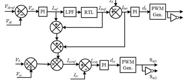
Fig. 7 Combined control for the proposed composite energy storage system.
