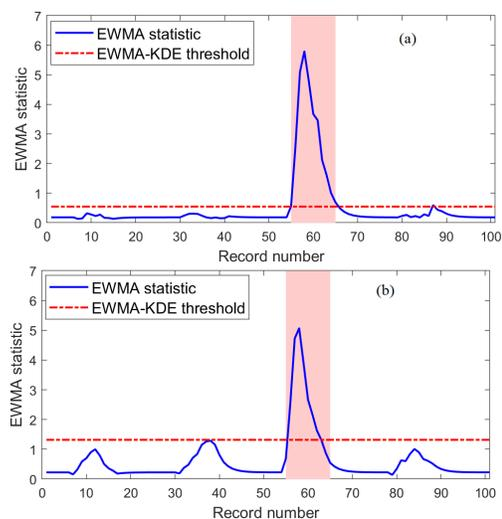
Fig. 5. Detection results of (a) BT-EWMA, and (b) BS-EWMA schemes in the presence of Sensor fault in pyranometer.
