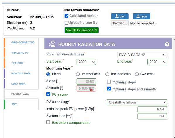
Fig. 1. PV system simulation via the PVGIS web-interface.
