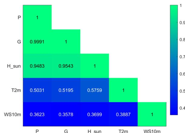
Fig. 2. Correlation matrix of input-output variables in a simulated PV system.
