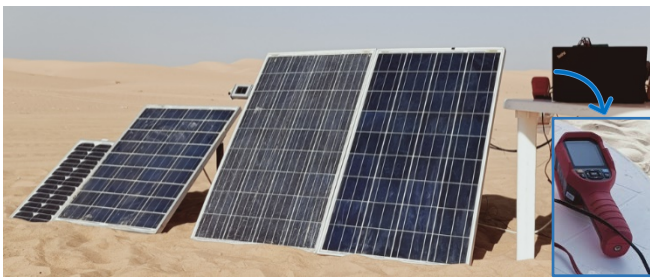
Fig.2 Test facility: the examined PV modules and IR camera
