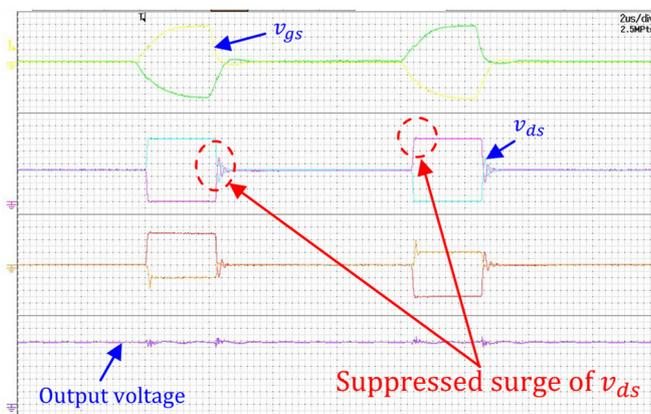
Fig. 9. Experimental switching waveforms of the half-bridge dc-dc converter using the proposed HB-PDEM.
