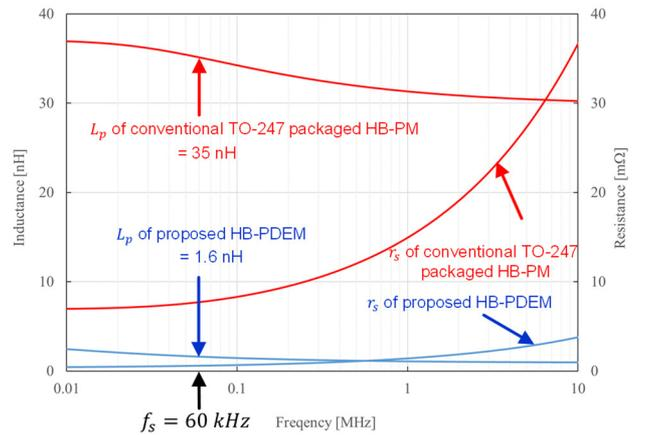
Fig. 5. Simulated parasitic inductances in the conventional TO-247 packaged HB-PM and the proposed HB-PDEM.
