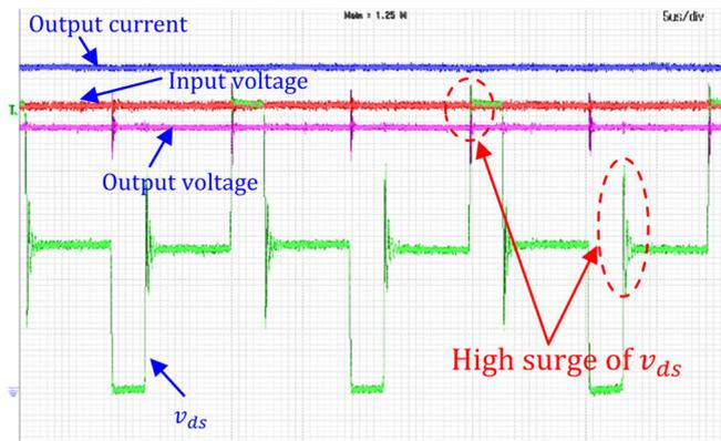
Fig. 8. Experimental switching waveforms of the half-bridge dc-dc converter using the discrete MOSFET.
