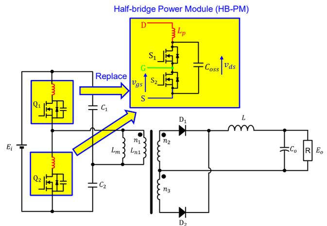
Fig. 1. Half-bridge dc-dc converter utilizing half-bridge power module (HB-PM).
