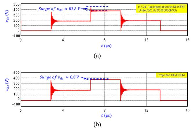
Fig. 6. Simulated surge of drain-to-source voltage comparison. (a) TO-247 packaged discrete MOSFET (UnitedSiC UJ3C065080K3S). (b) Proposed HB-PDEM.
