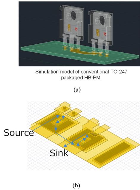
Fig. 4. Simulation models. (a) Conventional TO-247 packaged HB-PM. (b) Proposed HB-PDEM.
