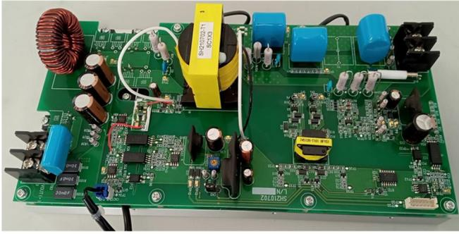
Fig. 7. 288 W prototype of the half-bridge dc-dc converter.
