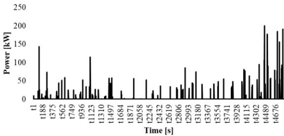
Fig. 5. Ultracapacitor discharge power variation.
