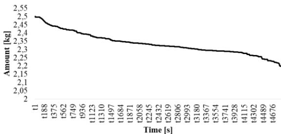
Fig. 4. The variation of total hydrogen amount in the tank.
