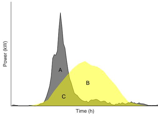
Fig. 2. Schematic outline of daily net load (A+C), net generation (B+C), and absolute self-consumed electricity (C) [7].
