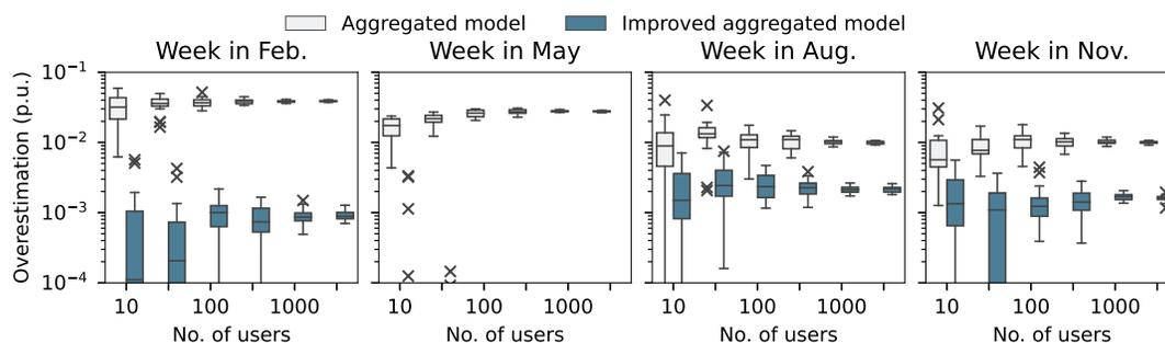
Fig. 8. Overestimation of the SCSB from both the original and the improved aggregated models. Note that the tick labels on the x-axis are only ordinal.
