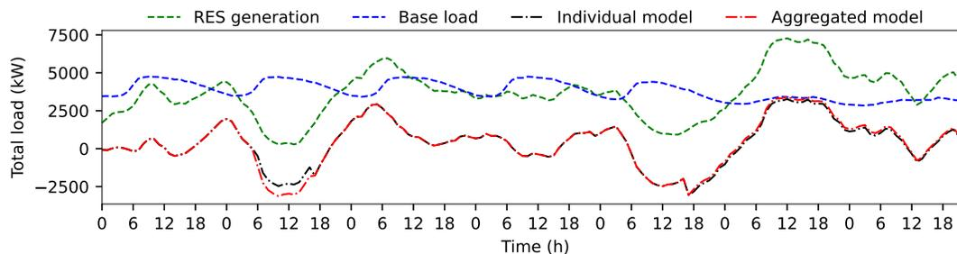
Fig. 7. The generation and load profile. The SCSB values for individual and aggregated models are 0.895 and 0.906.
