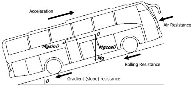
Fig. 2. Longitudinal Forces on a bus in motion.
