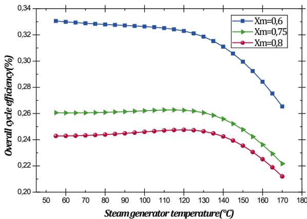
Fig. 3. The variation of the overall cycle efficiency as a function of the steam generator temperature for different mass fractions
