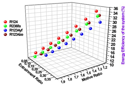
Fig. 8. Overall efficiency of the system as a function of the Entrainment ratio and the Motive ratio of the ORC Cycle
