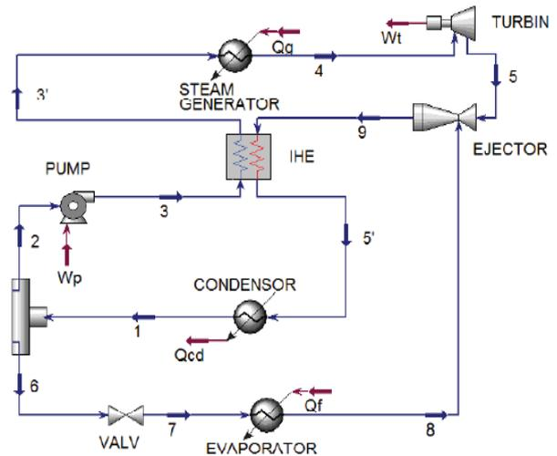
Fig. 2. Schematic of the ORC Cycle
