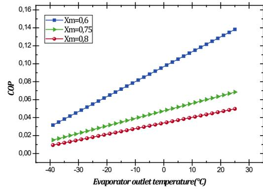
Fig. 4. Evolution of the coefficient of performance as a function of the evaporator temperature
