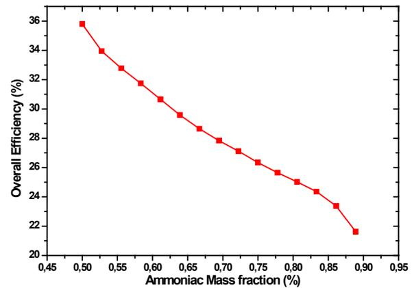
Fig. 5. Evolution of the Overall efficiency with ammonia concentration
