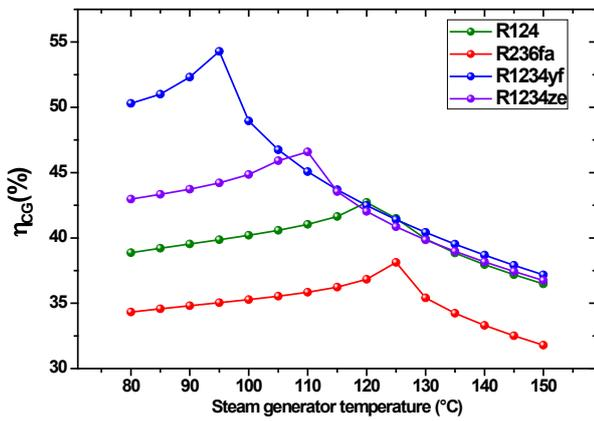
Fig. 6. Variation of the Overall efficiency of the ORC cycle as a function of the steam generator temperature
