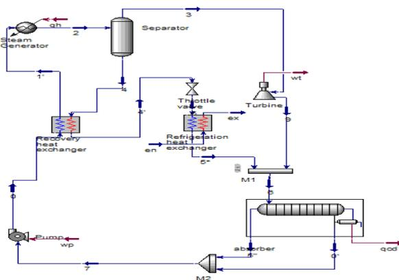
Fig. 1. Schematic of the Kalina Cycle
