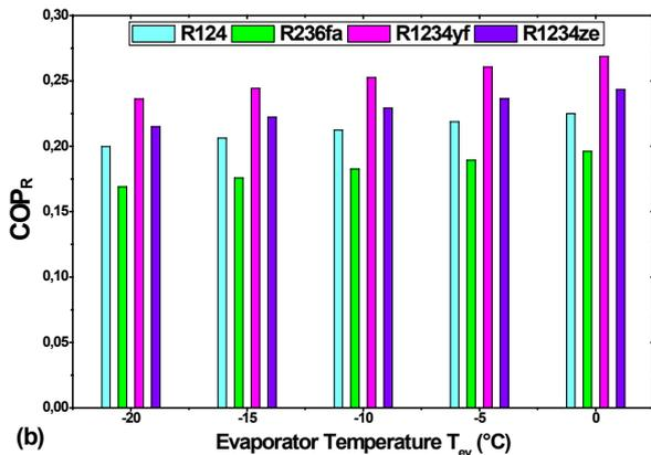
Fig. 7. Influence of the evaporator temperature on the refrigeration coefficient of performance of the ORC cycle
