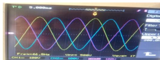
Fig. 15: Output of Three Phase 125 Level Inverter
