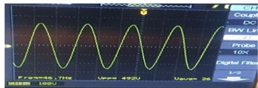
Fig. 14: Output of Single Phase 125 Level Inverter
