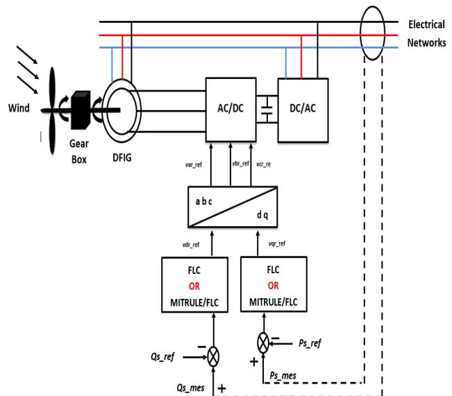
Fig. 1. Diagram blocs of the considered wind system.
