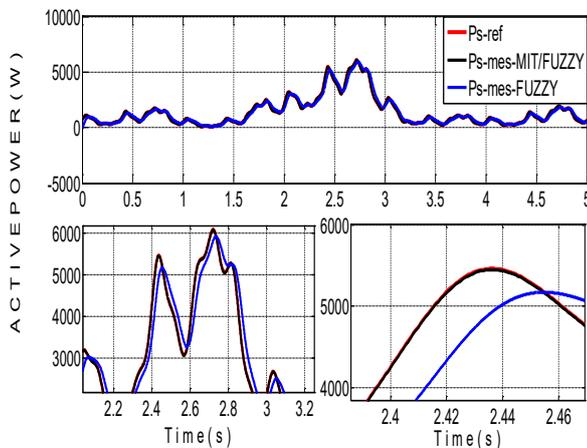
Fig. 11. Stator-active power in random wind speed
