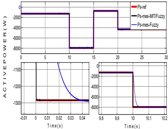
Fig. 8. Stator-active power after control and regulation
