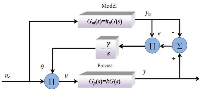
Fig. 3. Block diagram of gain in anticipation adaptation [10] [12].
