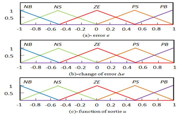
Fig. 2. Membership functions of: (a) error  $e$ ; (b) change of error  $\Delta e$ ; (c) function of sortie  $u$
