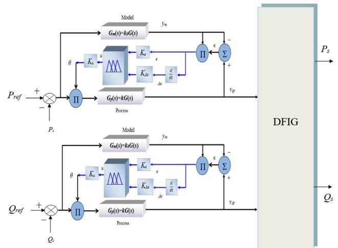
Fig. 4. Block diagram of active and reactive power control by MIT rule / fuzzy logic
