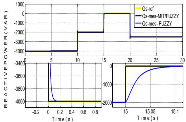
Fig. 9. Stator-reactive power after control and regulation
