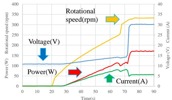
(c) 8-pole 12V, 4-pole 12V to 4-pole 24V.
