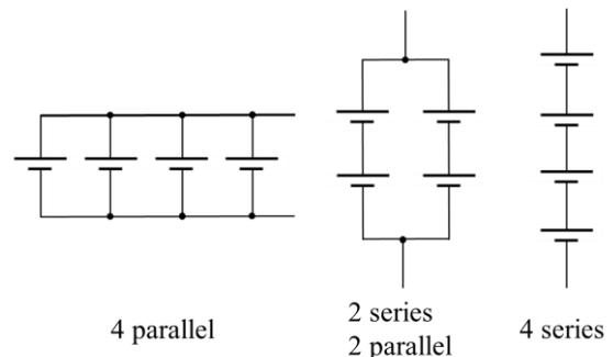
Fig. 2. Storage Battery Switching.
