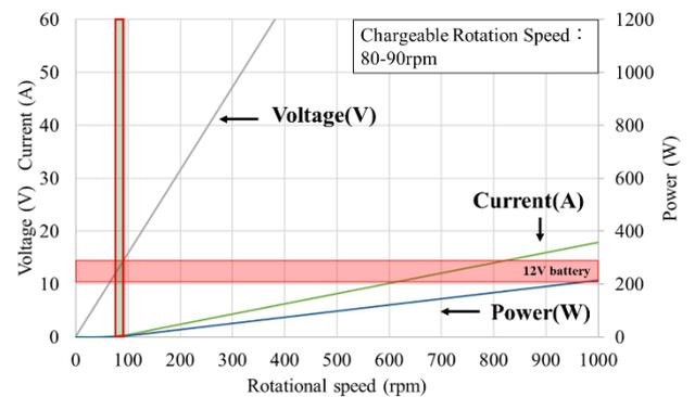
(a) Voltage, current, and power characteristics of 8-pole 12 V.
