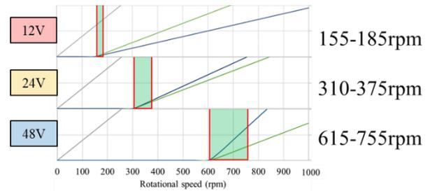
Fig. 5. Charging characteristics at 4-pole.
