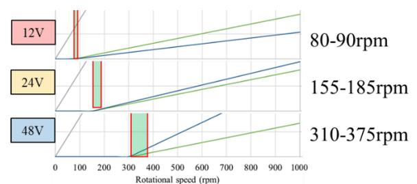
(b) Power generation characteristics at each battery voltage.
