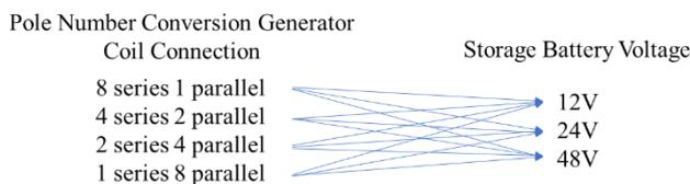
Fig. 3. Combination of number of generator poles and storage battery voltage.
