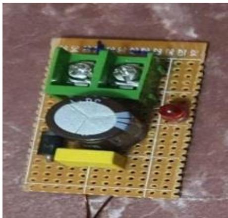
Figure 5. Real circuit of the IWPT system at the Rx side.
