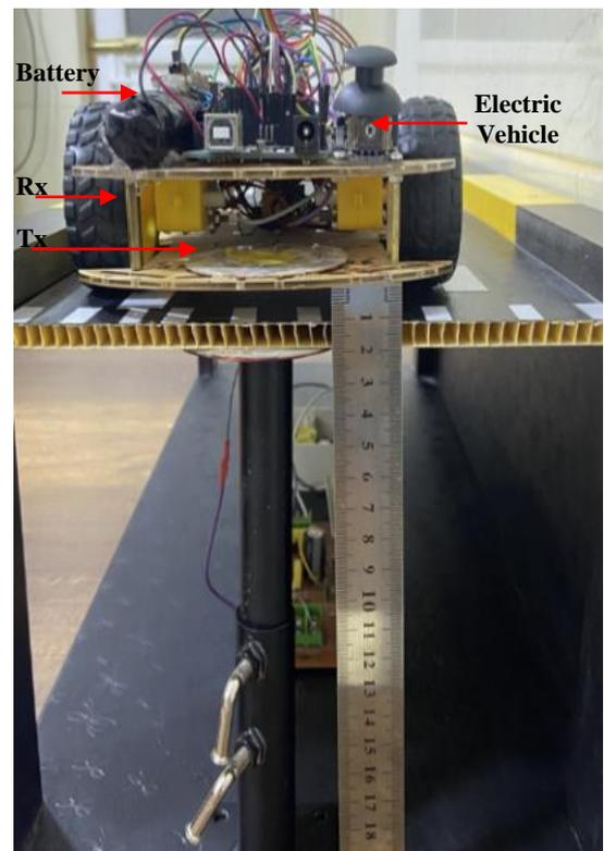
Figure 5. The implemented static charging IWPT prototype.
