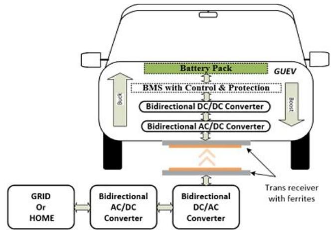
Fig. (1) Scheme of a static charging IWPT system for an electric vehicle [2].
