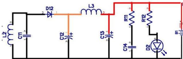
Figure 4. Schematic circuit of the IWPT system at the Rx side.
