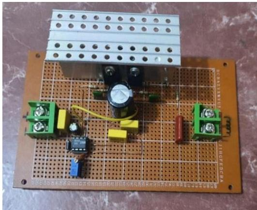
Figure 3. Real circuit of the IWPT system at the Tx side.
