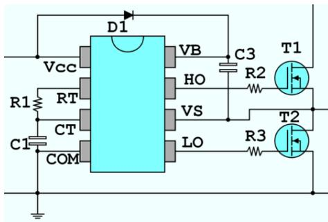
Figure 4. Circuit diagram of half-bridge driver (IR2153) for a Class-D inverter.
