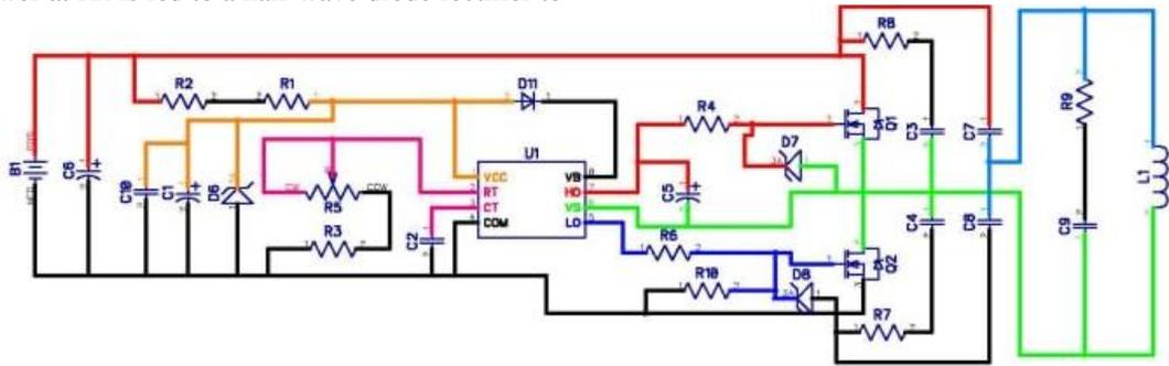
Figure 2. Schematic circuit of the IWPT system at the Tx side.
