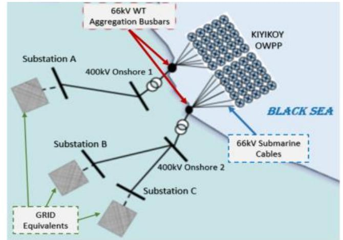
Fig. 2 Grid connections of the constructed system.
