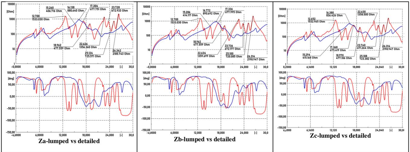
Fig. 5 Harmonic phase impedances seen at Substation A connection busbar for original and renewed states of Trakya grid (red line representing frequency sweep results for a all lumped grid scenario and blue line representing results for when the Trakya grid is modelled in detail
