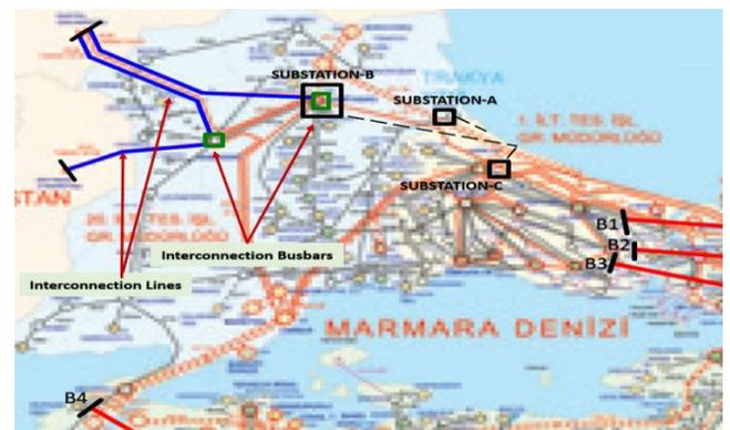
Fig. 1 Detailed modeled Trakya Region and its connections with the rest of the grid, B1, B2, B3 and B4 are boundary busbars representing Trakya side ending points of the connection lines over the Bosphorus and Dardanelles. Substation A, B and C are denoting three connection busbars of OWPP.
