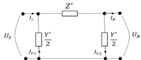
Fig. 3 Equivalent Pi model for transmission lines [2]
