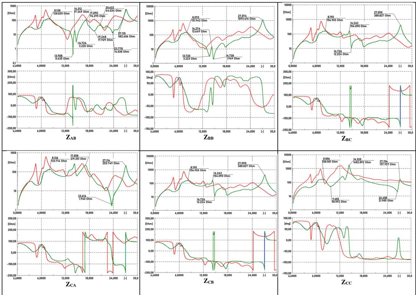
Fig. 6 Direct and transfer impedances for three PoC i.e.  $Z_{AA}$  is direct impedance for Substation A and  $Z_{AB}$  and  $Z_{AC}$  are transfer impedances between Substation A - Substation B and Substation A - Substation C respectively. Each graph is given with an additional impedance angle graph at the bottom and
