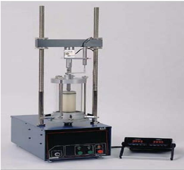
Fig 2. Versa Loader ASTM D1883.
