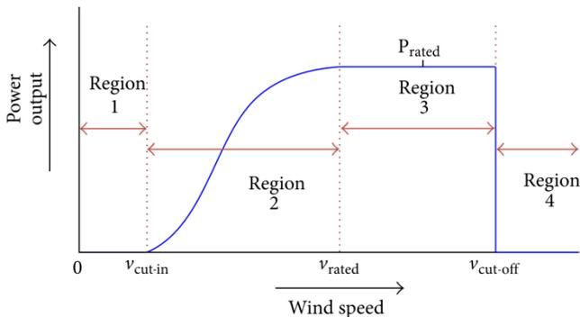
Fig. 1. Operating regions of a wind turbine power curve [9]
