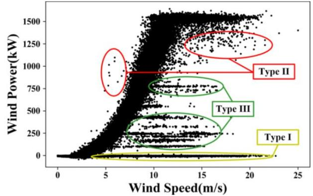
Fig. 2. Outlier types in a wind turbine power curve [12]
