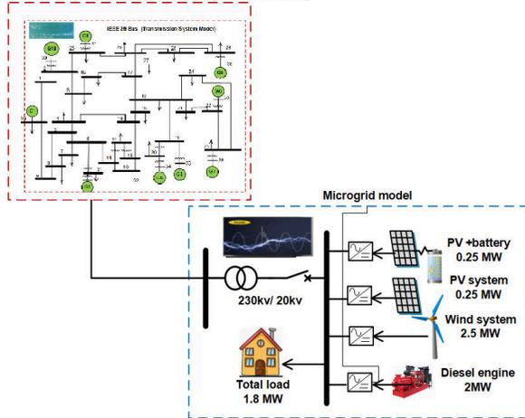
Fig.1 Schematic diagram of the integrated microgrid
