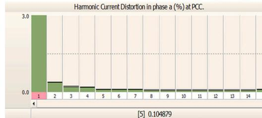
Fig.7 Individual harmonic distortion (%) of the current in phase a at PCC
