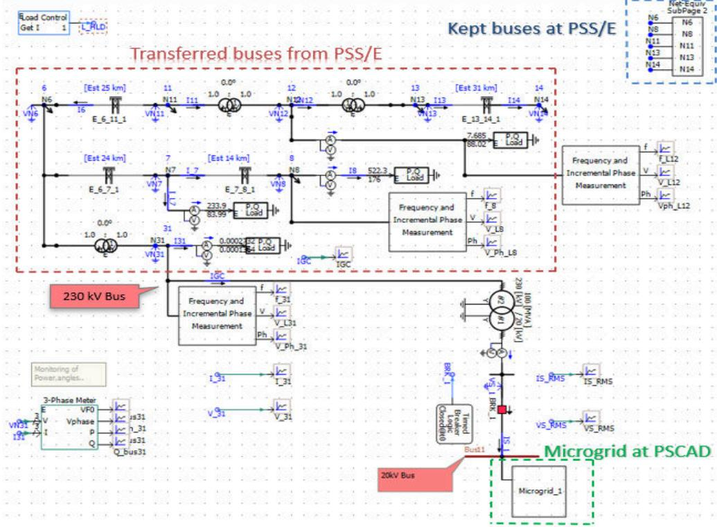
Fig.5 Transmission-Microgrid Co-Simulation Model
