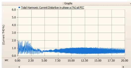
Fig.6 THD (%) of the current in phase a at PCC
