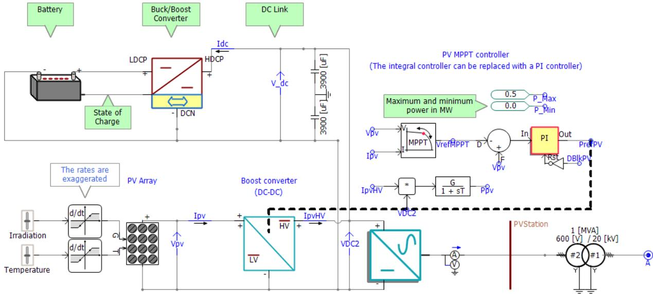
Fig.3 Solar photovoltaic with a battery storage
