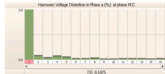
Fig.9 Individual harmonic distortion (%) of the voltage in phase "A" at PCC.
