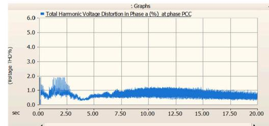
Fig.8 THD (%) of the voltage in phase a at PCC
